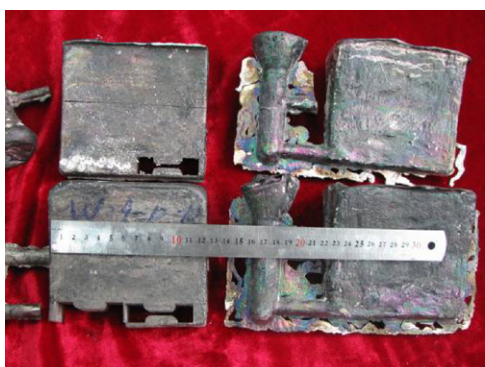
Fig. 2. Photo of the castings and gage dimension of rectangle tensile specimen.
